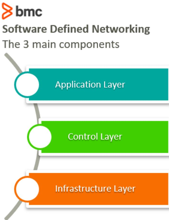
The major architectural differences between SDN and traditional network infrastructure are identified within the Control and Infrastructure layers. However, it is the SDN programs within the Application layer that define the new approach of data communication between controllers and services that run over the network.
